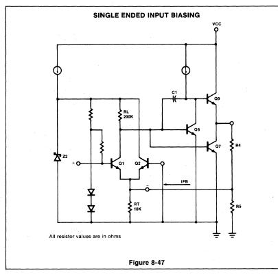
For bias stability, the current through R5 is made ten times the input current of Q2 ( $\approx 0.5 \mu$ A). Then, for the differential input, resistors R5 and R4 are:
