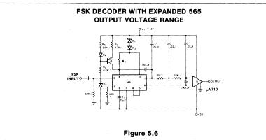
and 7 of the 565 and across the input of the comparator to avoid possible oscillation problems.
