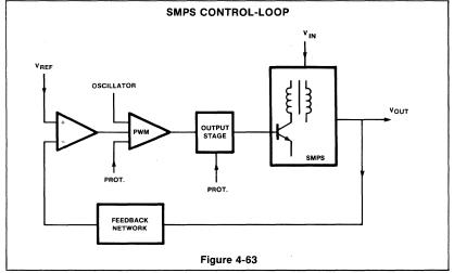
The other input of this modulator is used for an oscillator signal, which can be a sawtooth or a triangle.
