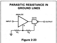
When the TTL gate output switches large ground currents occur on the gate ground leads. This transient current flows through R1 and R2, raising the voltage at points A and B. These potentials can cause positive (or negative) feedback which can alter the ideal transfer curve of Figure 2-24a to that of Figure 2-24b. Both discontinuities and hysteresis are evident.
