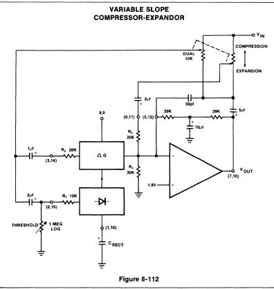
sion ratio is desired, proper selection of fixed resistors can be used instead of the potentiometer. The optional threshold resistor will make the compression or expansion ratio deviate towards 1:1 at low levels. A wide variety of (input) output characteristics can be created with this circuit, some of which are shown in Figure 8-113.
