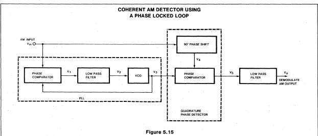
The low pass filter must remove all ac terms leaving only a dc voltage to drive the VCO. This must be the case for the analysis to be consistent with the assumption of Equation 5.15.
