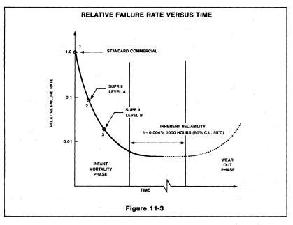
nated by the manufacturing control and preconditioning steps of SUPR II Level A processing. More persistent defects can be removed by the use of "burn-in" techniques. The "burn-in" processing of SUPR II Level B effectively allows the system manufacturer to ship his equipment at Point 3 on the failure rate curve in Figure 11-3.
