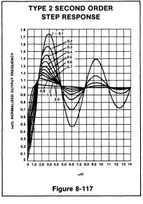
Figure 8-117 shows that the loop will settle to within 5% of its final value at  $\omega_{\rm N}T = 4.5$  if we use a damping factor of  $\alpha = 0.8$ . The required lock-up time was arbitrarily chosen to be 50 ms.
