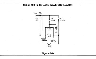
A single section of the Quad time may be used as a non precision oscillator. The values given are for oscillation at about 400Hz. T<sub>1</sub>  $\approx$  R<sub>1</sub>C<sub>1</sub> and T<sub>2</sub>  $\approx$  2.25 R<sub>2</sub> C<sub>2</sub> for Vcc of 15 volts. The frequency of oscillation is subject to the changes in Vcc.
