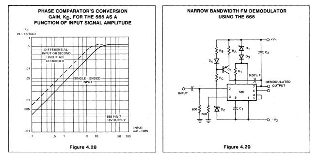
rent can be varied only a small amount due to the small change in current through R<sub>1</sub>. Consequently, the VCO can track the input signal over a small frequency range yet the output voltage of the loop (control voltage of the VCO) will swing its maximum value.
