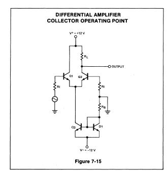
signal relative to ground, the collector operating point must be made more positive to allow for the common mode input signal if nonsymmetrical distortion is to be eliminated. For example, if the input signal is 10mV peak-to-peak riding a 2V common mode signal, the collector operating point must be raised according to the following equation:
