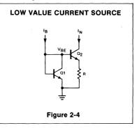
If the geometries of Q1 and Q2 are identical, the following equations hold:
