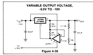
**NEGATIVE OUTPUT VOLTAGE CIRCUIT**  $\downarrow \mu 77000 ^{2} _{\mu A77000} ^{2} _{\nu A7700} ^{2} _{\nu A7700}$
