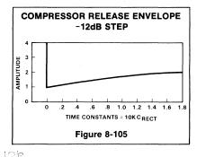
prevent C<sub>4</sub> from becoming completely discharged. The gain cell is activated when the voltage on pin 1 or 16 exceeds two diode drops. If C<sub>4</sub> were allowed to completely discharge, there would be a slight delay before it recharged to > 1.2V and activated limiting action.
