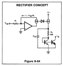
negative or positive signal swings, respectively. IC's such as this have typical npn  $\beta$ 's of 200 and pnp  $\beta$ 's of 40. The  $\alpha$ 's of .995 and .975 will produce errors of .5% on negative swings and 2.5% on positive swings. The 1.5% average of these errors yields a mere -13dB gain error.
