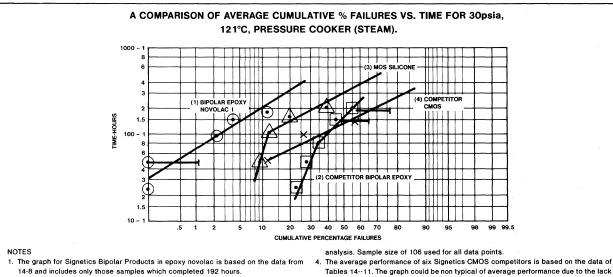
2. The average performance of competitor bipolar products in epoxy is based on the data of Table 14-9 and a sample size of 203 through 192 hours
