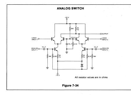
application. In the application of the 511, the user is cautioned to maintain short leads and maintain input/output isolation as the circuit transistors have gains in excess of unity at frequencies as high as 500MHz. The user should also note that the isolation contact substrate *must* always be connected to the most negative point of the circuit.
