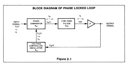
the system. The band of frequencies over which the PLL can acquire lock with an incoming signal is known as the "capture range" of the system and is never greater than the lock range.
