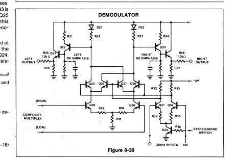
$$V_{out} = \left(\frac{V_e}{R21}\right) R_{ext}$$
