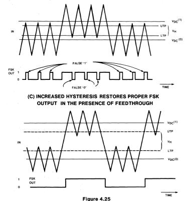
are less than the  $f_0'$  change with temperature. However this effect can be eliminated if the dc or average value of the amplifier signal is retrieved and used as the reference voltage for the Schmitt trigger. In this manner, variations in the  $f_0'$  with temperature do not affect the FSK output.
