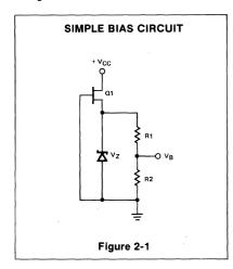
Zener  $V_Z$  is fed current by FET Q1. The required bias voltage is then developed by the resistor divider R1 and R2. This simple technique can be elaborated upon if temperature compensation is required. By adding transistor Q2 shown in Figure 2-2, the positive temperature coefficient of the zener diode is offset by the negative one of the forward biased emitter-base diode.
