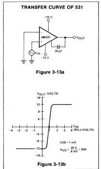
and +10 volts where it crosses the  $E_{in}$  axis, the voltage gain and offset voltage may be determined. It can be seen that the voltage gain of the device under test, (D.U.T.), is 50,000 and its input offset voltage is 1.0mV.
