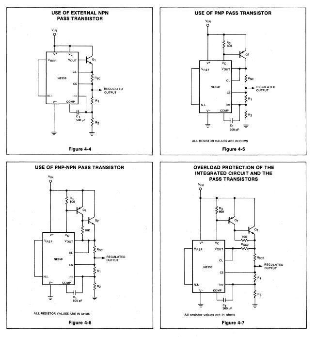
This arrangement has the merit of economy, since npn power transistors are generally cheaper than pnp, but has the disadvantage that the minimum differential voltage between input and output is increased by the  $V_{BEs}$  of the external transistors. The load regulation is also somewhat degraded since the error amplifier gain is finite and the  $V_{BE}$
