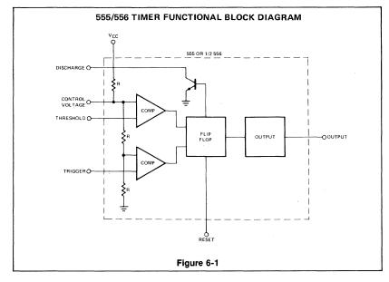
The resistive divider network is used to set the comparator levels. Since all three resistors are of equal value, the thresholo comparator is referenced internally at 2/3 of supply voltage level and the trigger comparator is referenced at 1/3 of supply voltage. The outputs of the comparators are tied to the bistable flip-flop. When the trigger voltage is moved below 1/3 of the supply, the comparator control of timing and oscillation functions is also available,
