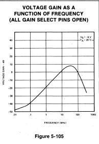
determine the voltage gain as a function of frequency.
