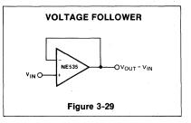
However, for most applications a direct connection from output to input will suffice. Errors arise from offset voltage, common mode rejection ratio and gain. The circuit can be used with any op amp with the required unity gain compensation, if it is required.
