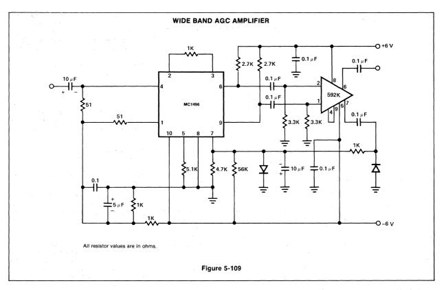
84, the signal is fed to the signal input of the MC1496 and RC coupled to the NE592. Unbalancing the carrier input of the MC1496 causes the signal to pass thru unattenuated. Rectifying and filtering one of the NE592 outputs produces a dc signal which is proportional to the ac signal amplitude. After filtering this control signal is applied to the MC1496 causing its gain to change.
