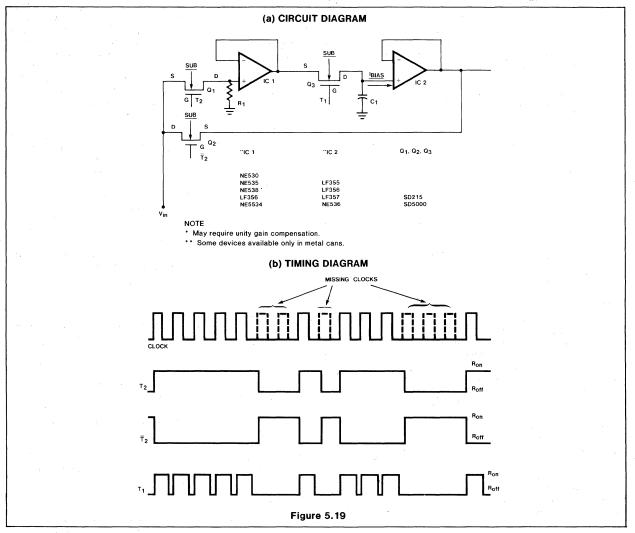
therefore the periodic "bit rate", is constant. For detection and further processing of the digits it is necessary to have a "clock" that is coherent with the bit rate. This clock must ordinarily be derived from the incoming data stream. Phaselock techniques are widely used to recover the clock from the data (11).
