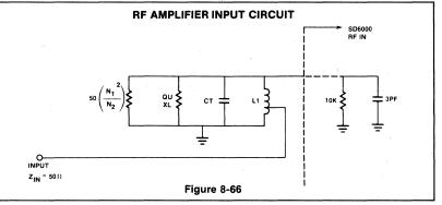
C<sub>P</sub> is made up of the D-MOS input, and a fixed parallel capacitor. The required C<sub>P</sub> is given by  $C_{P} = \frac{1}{(8-32)}$
