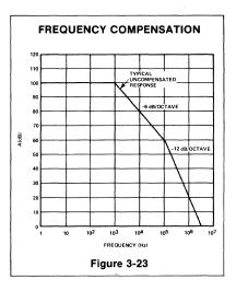
gain of the amplifier is greater than one for the frequency at which the 180° phase shift is reached. By adding poles and zeros to the amplifier response externally, the phase shift can be controlled to insure stability.
