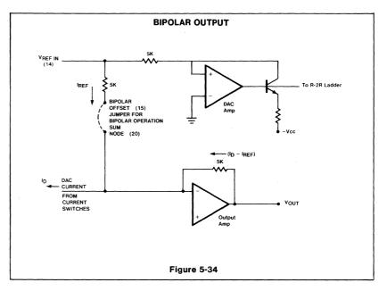
current output structure allows the user to provide a programmable current sink ( $I_{OUT}$  max of 2mA). Several jumper options provide a variety of operational modes. Figure
