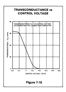
is at the discretion of the user. This allows the circuit designer complete freedom of choice in operating parameters and transistor interconnections. The only constraints are the absolute maximum ratings of the device; for example, applied voltage, current, junction temperature, etc.
