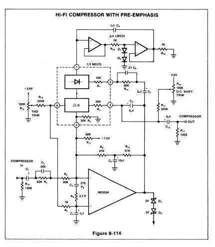
Both the compressor and expandor have unity gain levels of 0dBm. Trim networks are shown for distortion (THD) and dc shift. The distortion trim should be done first, with an input of 0dBm at 10kHz. The dc shift should be adjusted for minimum envelope bounce with tone bursts. When applied to consumer tape recorders, the subjective performance of this system is excellent.
