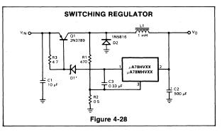
collector voltage starts to decrease and the positive feedback loop completes the switching action.
