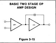
feedback configuration, this implies an open loop gain of unity at this frequency. The capacitor  $C_c$  controls this parameter by looking much smaller than  $r_m$  at frequencies above a few cycles, giving a clean 6dB/octave roll off over 5 decades.
