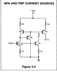
Assuming Q1-Q2 and Q4-Q5 are well matched and of the same geometries it can be shown that : Equations
