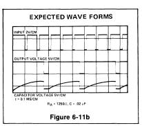
Figure 6-11b shows the waveforms of the timer in Figure 6-11a when used as a divide by three circuit. This application makes use of the fact that this circuit cannot be retriggered during the timing cycle.
