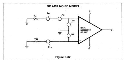
transistors. These noises are included in  $E_{\mbox{\scriptsize N}},$  the total equivalent input voltage noise generator.
