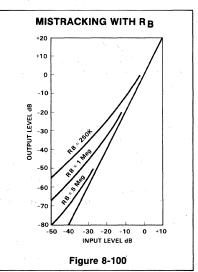
expandor gain will stop dropping and the expansion will cease. In a compressor this would lead to a lack of compression at low levels. Figure 8-100 shows some typical transfer curves. An  $R_b$  value of approximately 2.5Meg would trim the low level tracking so as to match the Bell system N2 trunk compandor characteristic.
