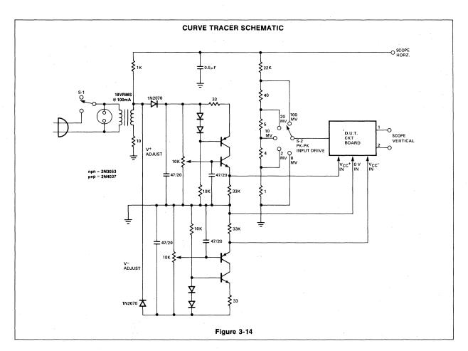
Simplicity and low cost are the two major attributes of this tester. It is not intended to perform highly rigorous tests for all devices. It is, however, a reasonably accurate means of determining the gains and offset voltages of most amplifiers. It will in addition, indicate the transfer curves of comparators and sense amplifiers with equivalent accuracies.
