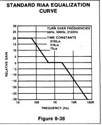
Magnetic types, however, produce small voltages in the neighborhood of 5mV and require preamplification.
