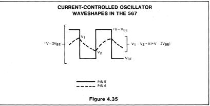
duty cycle by drawing  $l_C$  of 100 $\mu A$  for the  $R_{2,1}$ , Q20 junction. When  $l_C$  is then varied between 0 and 200 $\mu A$ , the frequency changes by  $\pm$ 7%. Because of the slight shift in the voltage levels  $V_1$  and  $V_2$  with  $l_C$ , the square wave duty cycle changes from about 47% to about 53% over the control range. To avoid drift of free-running frequency with temperature and supply voltage changes when  $l_C \neq$  0,  $l_C$  is also made a function of +V - 2 VBE.
