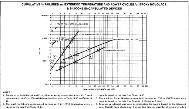
3. The graph for Epoxy Novolac encapsulated devices vs. 0 to 125°C temperature cycle is based on the data from Table 5-13 through 7000 cycles.
