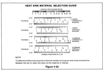
To determine the thermal resistance of a heat sink, subtract the junction-to-case thermal resistance,  $\Theta_{JC}$ , of the selected package from the Line E intersection.
