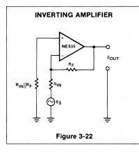
As opposed to the non-inverting circuits the input impedance of the inverting amplifier is not infinite but becomes essentially equal to R<sub>in</sub>. This circuit has found widespread acceptance because of the ease with which input impedance and gain can be controlled to advantage, as in the case of the summing amplifier.
