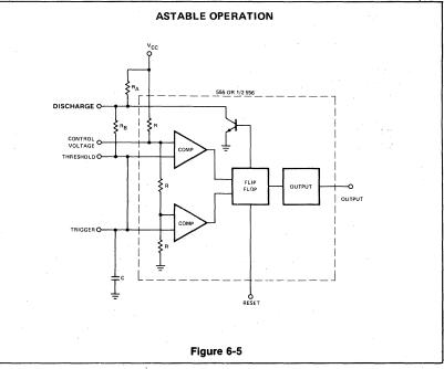
drives the output low and turns on the discharge transistor. The transistor discharges the capacitor, C, rapidly. The timer has completed its cycle and will now await another trigger pulse.
