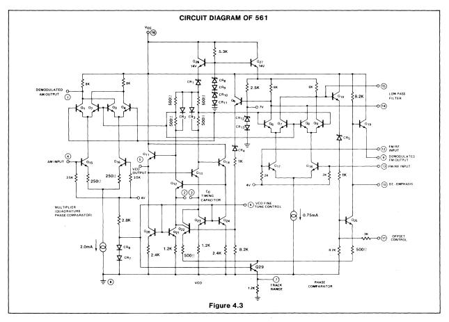
rather than differential (as the loop phase comparator input), and an external 90° phase shift network is required to provide the proper phase relations. The demodulated AM output is brought out at pin 1.
