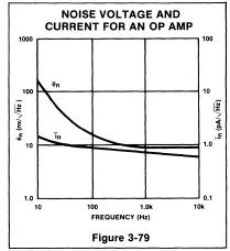
noise voltage which is in x  $R_{in}$  (or  $X_{cin}$ ). The output is measured, divided by amplifier gain, referenced to input, and that contribution known to be due to  $\overline{e}_n$  and resistor noise is appropriately subtracted from the total measured noise. If a capacitor is used at the
