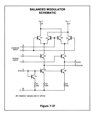
a low level signal, VS, driving the third differential amplifier Q5-Q6, the output voltage will be a full wave multiplication of  $V_C$  and Vs. Thus for sine wave signals, Vout becomes:
