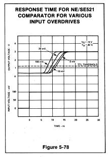
specified excess or overdrive signal. This causes the amplifier to be exercised from saturation in one direction to saturation in the other for worst case propagation delay. Note that larger overdrive improves delay time as can be seen in Figure 5-78. An overdrive of 5mV causes 12ns delay, whereas a 100mV overdrive improves transit time to only 6ns.
