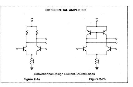
vantages of the circuit in Figure 2-7b are that the noise in the pnps is summed into the npn input noise, and the self-biasing scheme used in Figure 2-7b can introduce some added offset current if the pnp betas are low because pnps run at different current levels. A change in the circuit which avoids this problem is shown in Figure 2-8. to the pnp emitters to increase the output impedance and, therefore, the gain.
