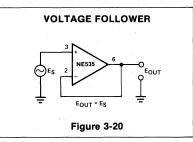
Applying the zero differential input theorem the voltages of pins 2 and 3 are equal and since pins 2 and 6 are tied together, their voltage is equal; hence,  $E_{out} = E_{in}$ . Trivial to analyze, the circuit nevertheless does illustrate the power of the zero differential voltage theorem. Because the input impedance is multiplied and the output impedance divided by the loop gain the voltage follower is extremely useful for buffering voltage sources and for impedance transformation.
