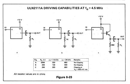
The final component required is a small decoupling capacitor placed between the network and the low amplifier output. To insure linear detector operation, the reactance of this capacitor should be substantially large, as compared to the impedance of the tuned circuit at resonance.
