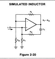
The Q of this inductance depends upon R1 being equal to R2. At this point the Q of the inductor is maximum. At the same time, however, the positive and negative feedback paths of the amplifier are equal leading to the distinct possibility of oscillation at high frequencies. R1 should therefore always be slightly smaller than R2 to assure stable operation.
