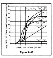
By definition the transconductance, gm is the partial derivative of drain current,  $i_d$ , with respect to the input voltage  $e_s$ . The total drain current of the mixer can be expressed by
