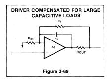
With large holding capacitors, an isolation resistor should be used between the input to the FET amplifier and the holding capacitor. This resistor prevents excessive input currents to the amplifier during power shut downs with a full charge on the capacitor.
