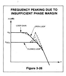
It is generally accepted in the interest of minimized frequency peaking to limit the phase shift of the amplifier to 135° or a phase margin of 45°. At this margin the second order response of the system is critically damped and oscillation is prevented.
