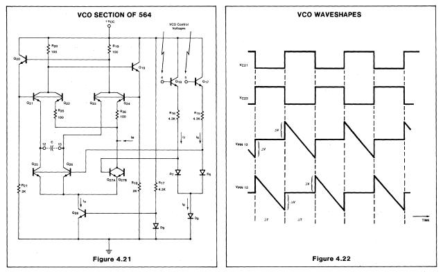
Q17 - Q18 and R<sub>15</sub> - R<sub>16</sub>, the VCO control voltage is applied differentially to the base of Q27 and to the common bases of Q25 and Q26.
