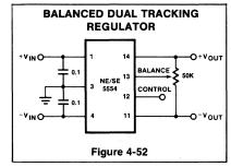
This output balance control may be used to change the positive regulated voltage from about 0.2 volts to  $\geq$  16 volts without changing the negative regulated voltage.
