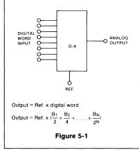
quantity; a set of binary switches to simulate binary coefficients  $B_1 \ldots B_N$ ; a weighting network; and an output summing means.
