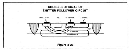
locating the resistor out of the transistor current path.
