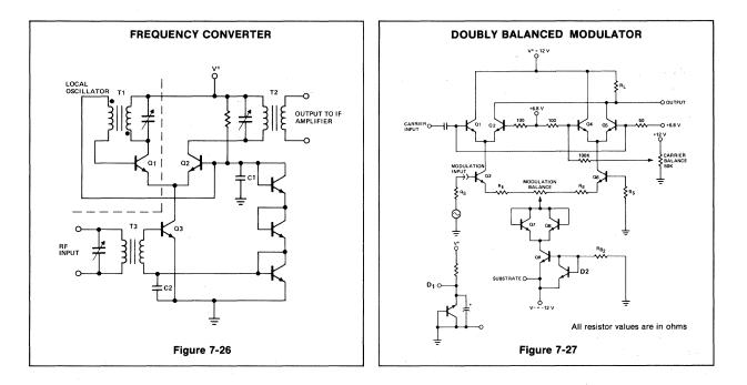
resistor is properly adjusted and with no modulation input, no carrier will be present at the output. When a modulation signal is impressed, the collector RF currents of the differential pair of transistors will be unbalanced and a RF signal will be present at the output, the phase of which will depend upon whether the modulation input is positive or negative.
