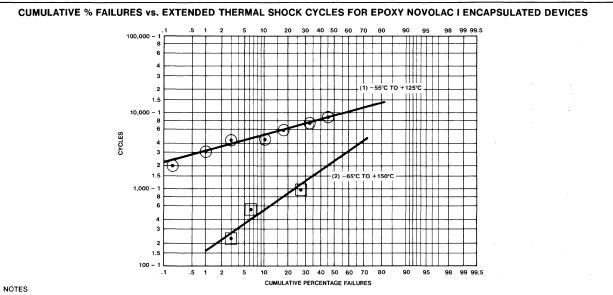
1. The graph for Epoxy Novolac encapsulated devices vs. -55°C to +125°C thermal shock is based on the data from Table 14-17 using the 8000 cycle sample size of 498.
