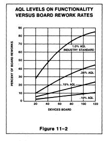
manufacturer has various options to solve problems arising from infant failures. He can ship his system to the end customer and repair field failures as they occur. He can operate the system in-house for this period and repair failures. Or he can purchase devices which have already been preconditioned to eliminate the early failures. Each customer must choose the most cost-effective method for his particular business. A alderable sumber of the vellability
