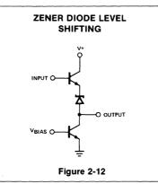
Multiples of this value can be gained by cascading more diodes. The benefits of this method are speed and small die area, while disadvantages include inflexibility to power supplies and high noise. These drawbacks restrict the use of this method to switching circuits such as comparators and sense amolifiers
