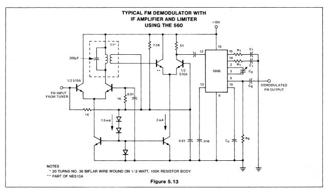
Implementation of the low pass filter can be made in either of two ways. The series combination of  $R_1$  and  $C_1$  connected to pins 14 and 15 as shown in Figure 5.13 uses  $R_1$  and  $C_1$  to set the bandwidth (in Hz) of the demodulated information according to
