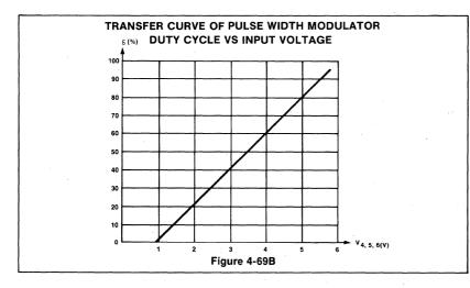
graph is given in Figure 4-69B. The output of the PWM causes the resetting of the output bistable.
