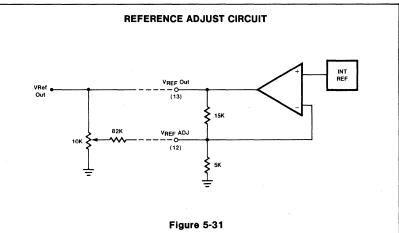
source. Compensation is required, when operating from a high impedance source. The addition of an external resistance reduces the phase margin of the amplifier making it less stable. Compensation, when required, is a single capacitor from pin 16 to ground.
