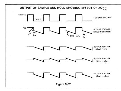
error for only one set of conditions. Figure 3-67 shows the comparative effects of C for different hold voltages. Because of this charge effect, the holding capacitor should be as large as possible for the desired sampling time. With a holding capacitor of  $.1\mu$ F this error is only .45mV.
