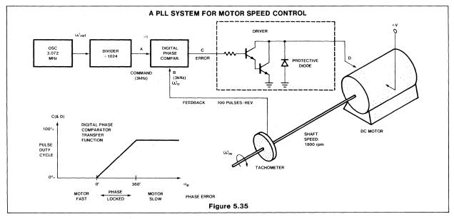
gate light pulses to phototransistors. Another way is to use variable reluctance coil pickups to sense gear teeth going past. Whatever principle is used, the tachometer should be made with precision or it will introduce noise and jitter into the system. It is recommended that this component be obtained from a company specializing in tachometers.
