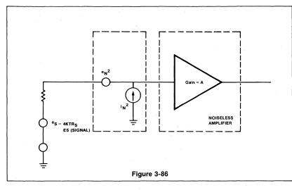
An amplifier gain of 68dB yields an output signal voltage of 1V rms.
