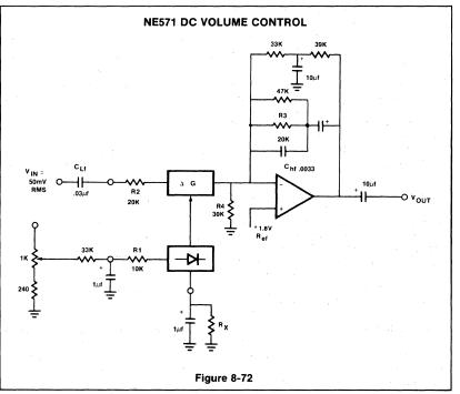
level control (ALC) circuit. The ALC circuit has a transfer function which makes its output voltage constant with a wide range of input levels. It is generally desirable to have an audio compressor which provides an output level which drives the modulator to close to 100% modulation with very low input levels and does not exceed 100% with large inputs.
