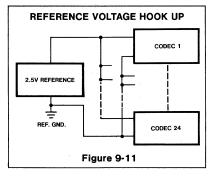
The presence of a separate reference ground helps to reduce any interference due to noise. The accuracy of the reference should be  $2.5V \pm 0.25\%$  with a temperature coefficient of  $\pm 10ppm/^{\circ}C$  to meet the specifications over a temperature range of 0°C to 70°C. The ST135 meets these requirements.
