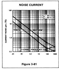
noise density plots such as in Figure 3-80 and 3-81. Above a certain corner frequency, white noise dominates; below that frequency, flicker (I/f) noise is dominant. Low noise corner frequencies distinguish low noise op amps from general purpose devices.
