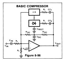
The same restrictions for the rectifier and  $\Delta G$  cell maximum input current still hold, which place a limit on the maximum compressor output. As in the expandor, the rectifier and  $\Delta G$  cell inputs could be made common to save a capacitor, but low level tracking accuracy would suffer. Since there is no dc feedback path around the op amp through the  $\Delta G$  cell, one must be provided
